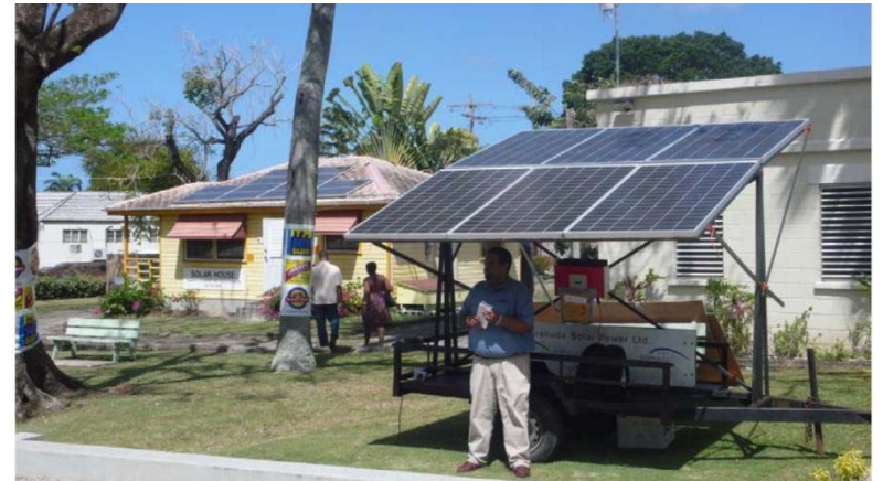
Exhibition in Barbados – Solar House and transportable grid-connected PV System (Photo credit: Grenada Solar Power Ltd. – Grensol)
